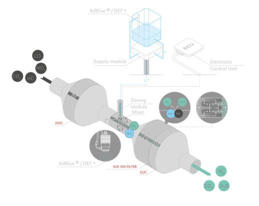
1. Diesel **Oxidation Catalyst**  $NO \rightarrow NO_{2}$ HC, CO and PM oxidation
